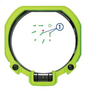
4 Using a 7/64 inch hex wrench, adjust the curved vertical @ and curved horizontal @ adjustments on the mount in the directions the arrows indicate. For example, if the arrows point up and right, move the curved mount pieces up and right.
